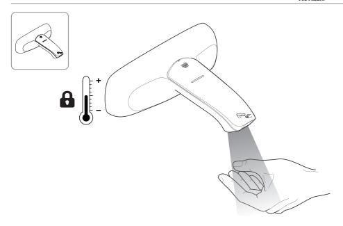
**Note:** This tap has an over temperature limiting device, should blend temperature exceed safe conditions, the valve will shut down and reset automatically once temperature returns to a safe state.
