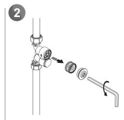
Unscrew and remove the filter.
