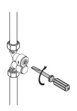
Turn the screw fully clockwise to isolate the water supply. Relieve the pressure by operating the tap.
