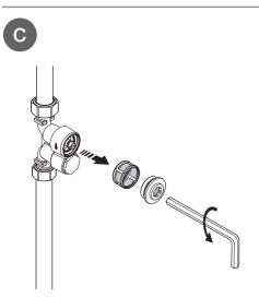
Using a 10 mm hexagonal wrench, unscrew and remove the filter.
