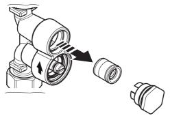
Remove the combined flow regulator / check valve and replace.
