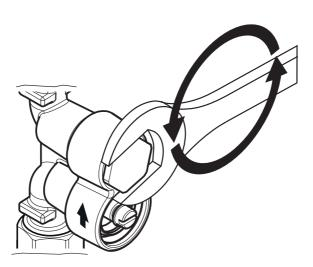
Using a suitable spanner, remove the check valve housing.
