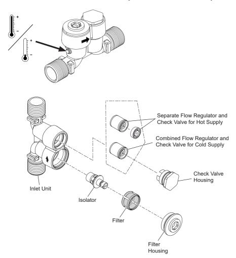
Filter contained in the unit is a fine 150 micron stainless steel mesh.
