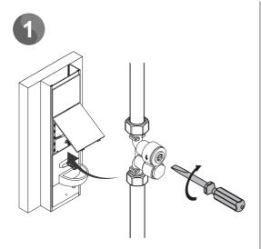
Turn the screw fully clockwise to isolate the water supply.
