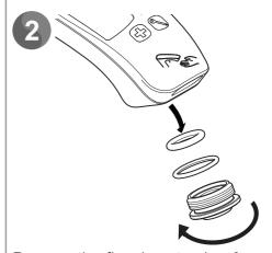
Remove the flow insert using 8 mm hexagonal wrench.
