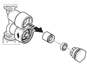
Remove the flow regulator and check valve. Make a note of the orientation of these components, this is critical to the unit operation.
