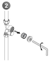
Unscrew and remove the filter.
