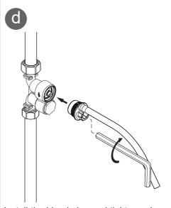
Install the bleed pipe and tighten using a 10 mm hexagonal wrench.
