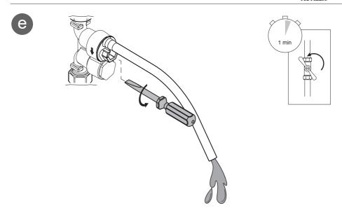
Using a suitable screwdriver, unscrew the screw to bleed the supply pipework.
